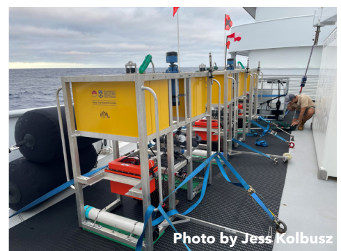
Photo by Jess Kolbusz Figure 1: Landers on deck ready for autonomous missions at the seafloor. These are released from the surface, sink to the bottom at a speed of 50-60 m/min. After landing, they carry out their mission at the bottom. They are recovered again by releasing a weight so that they rise the surface where they are recovered.
