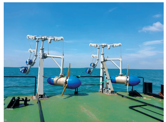
Figure 2: Turbines hoisted out of the water for maintenance.
