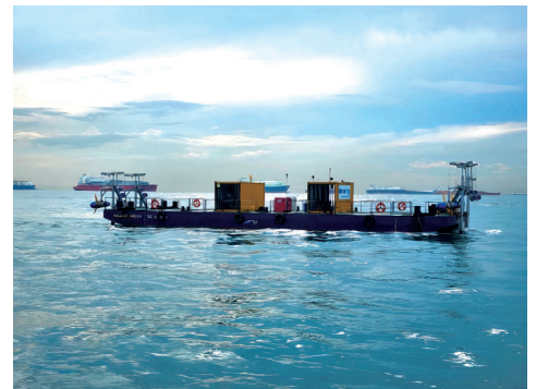
Figure 1: Floating barge with turbines anchored at both ends for generating electricity.
