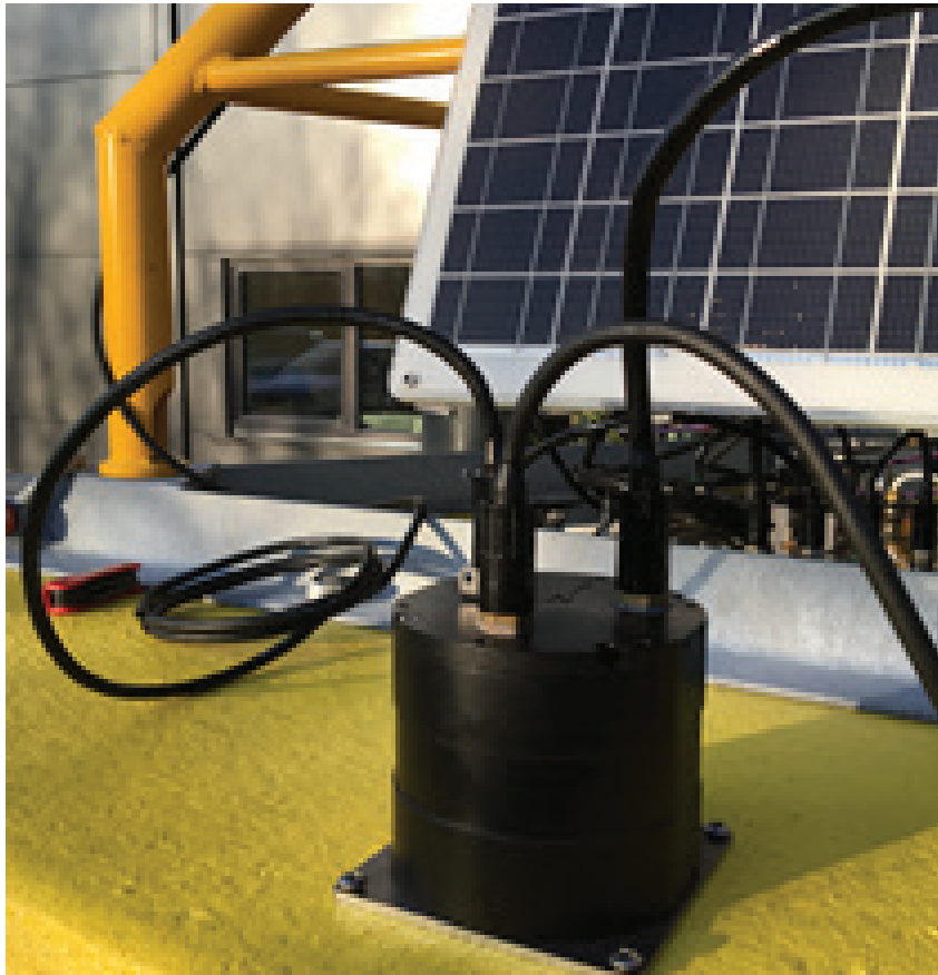
Figure 4: One of the MOTUS sensor was mounted about 50cm off-center on an EMM 2.0 buoy and another in the center.
