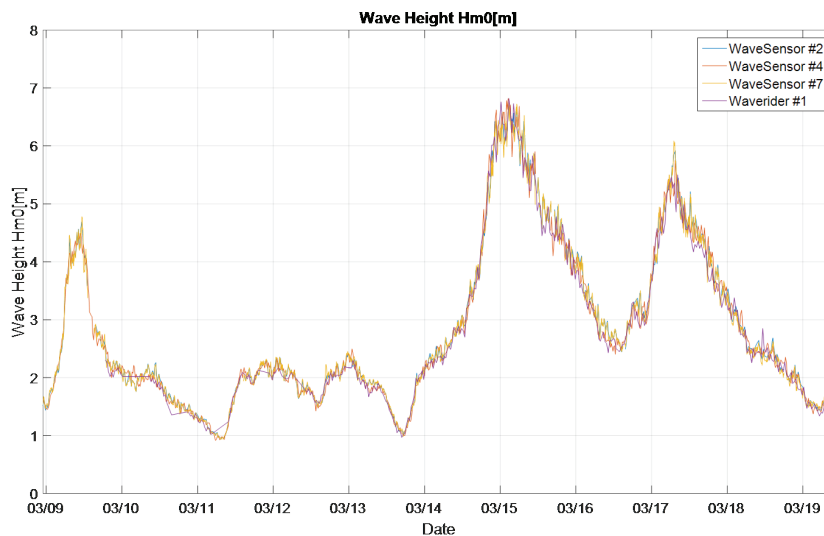
Figure 8: Significant wave height (Hm0) from Waverider (purple) and three MOTUS sensors on the Navigational buoy (#4 orange, mounted in center) and on the Hydmet buoy (#7 yellow, 50cm off-center and #2 blue, in center).
