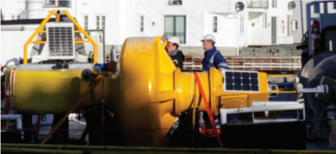
Figure 3: Picture of an YSI EMM 2.0 buoy (left) and a Tideland SB-138P navigational buoy (right) before being deployed at sea together with a Waverider buoy.
