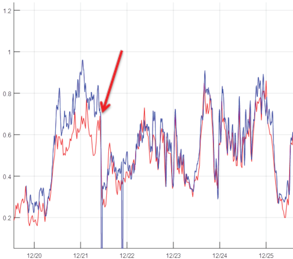
Figure 11: Significant wave height H_{m0} from a field test conducted at Bjørnafjorden December 2016. The red trace is from an offset installed MOTUS wave sensor on a Tideland SB-138P and the blue trace is from a Datawell Waverider. The red arrow marks the moment when the off-center compensation is switched on.
